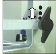
Adjust the speed, which is correct for the drill bit diameter, on the adjusting wheel and switch the machine on. Please decide in accordance with the information of the drill bit manufacturer.
