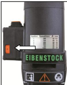
The machine is equipped with an adjusting wheel in order to allow a stepless speed control from 250 to 1000 rpm.
