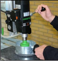
Put the tile or plate you want to drill on the drilling table and adjust it.
