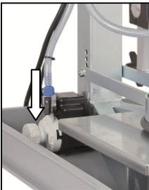
The **EFB 152 PX** has a water circulation by means of a pump. Before you start working with the machine, fill the pan with water until the suction connection is completely covered. This is the only way to assure a proper operation.
