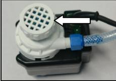
The pump is equipped with a filter sponge to protect it against dirty cooling water.
