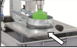
Use the cover plate for holes up to 40 mm in diameter. The cover plate must be removed for holes larger than 40 mm.
