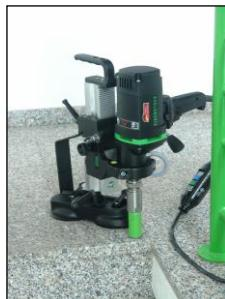
At the beginning, drill very slowly, since the drill bit does only starts cutting with a fraction of the cut surface in the material. If you drill too fast or with too much pressure, the drill bit could get jammed.
