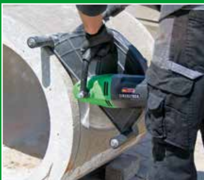
precise cutting depth adjustment (accessory)
