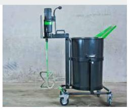
Drive unit with stirring rod can be separated from the carriage without any tools
