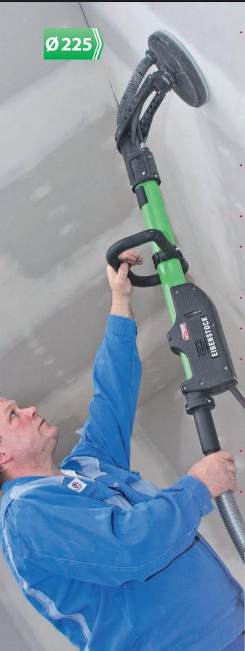
Spring-mounted suction hood with sealing lip VacuGlide
