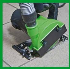
Joint milling – dry cutting with depth limiting and immersion function
